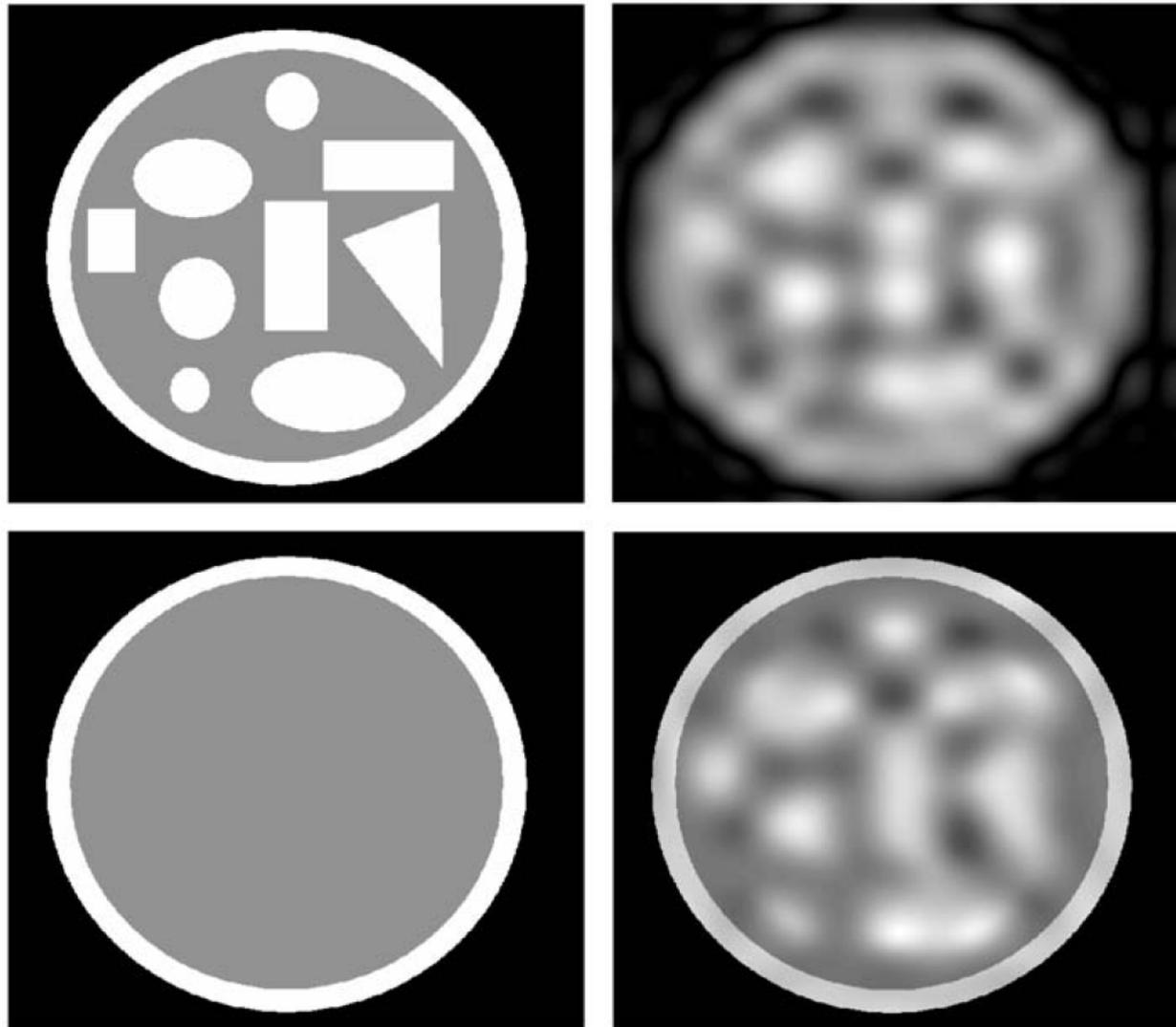
Reconstruction (bottom-right) of a test object (top-left) function from band-limited data (top-right) using prior information (bottom-left).
